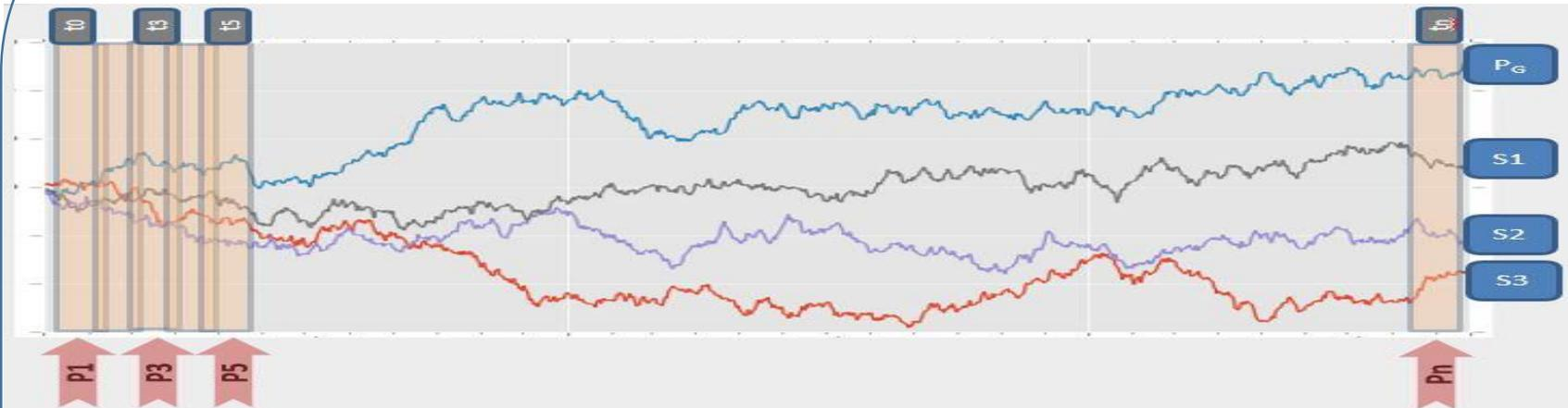
Visual Analysis of Patterns detected out of the sensor data and visual detection of transition patterns that identify degradation towards failure of the system
